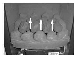
c) Fit the remaining three coals onto the ribs in the fuelbed as shown below, ensuring that the rear flame paths as indicated are not interupted See Fig. 22 below.
